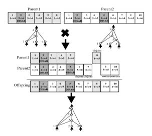
Our current approach to solving self-driving cars in a simulated environment relies on leveraging NEAT algorithms to iteratively search for the best architecture for the current environment. There is a set of cars that are generated in each
